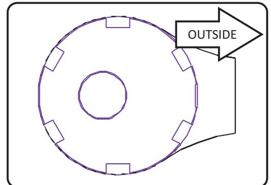
Fig 1. Maximum positive camber setting.
