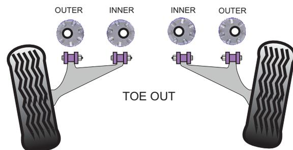
Hole positions in the sleeves, looking at them from the outside of the car on both sides, showing maximum adjustment limits. The adjusters will have to be adjusted individually to achieve the desired toe and camber settings.
