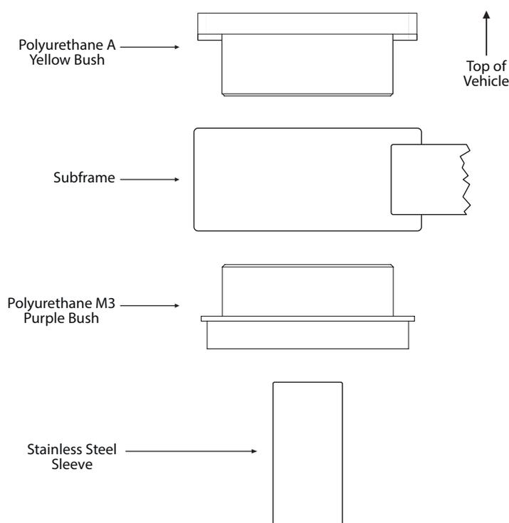
Figure 1: Exploded Assembly
