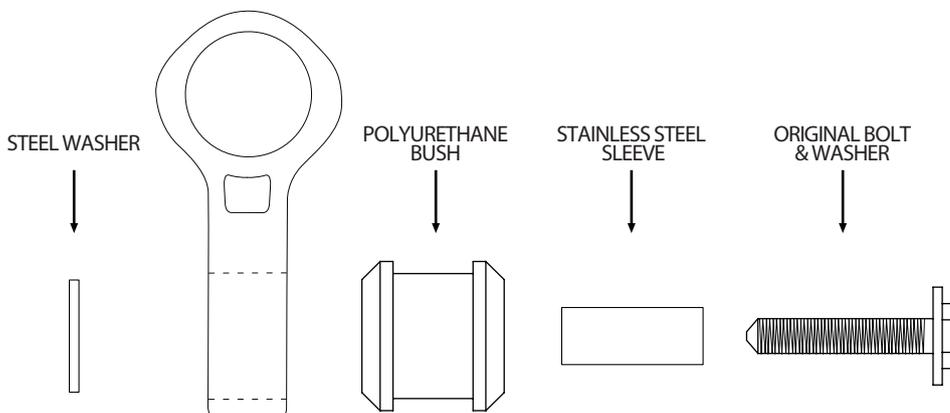
Figure 1: Assembly exploded view
