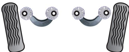
Sleeves adjusted to give maximum positive camber
