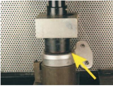
FIT OUTER PART INTO HOUSING SQUARE WITH PRESS, TAPER END FIRST CHECK CORRECT WAY ROUND
