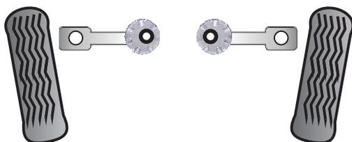
Sleeves adjusted to give maximum positive camber
