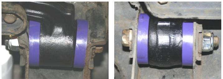
PFF27-302 – front upper wishbone bushes installed. Ensure that the smaller diameter washer is placed towards the inside of the wishbone and the larger diameter washer is placed towards the outside of the wishbone as shown in the diagrams.
