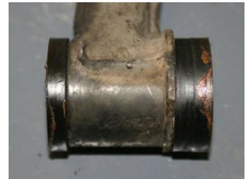
PFR17-209 fitted similar to PFF17-201. It is important to retain the original heatshield and re-apply it after fitting the POWERFLEX bush. If the original heatshield is no longer present, ensure a replacement heatshield is fitted. Note washer locations.
